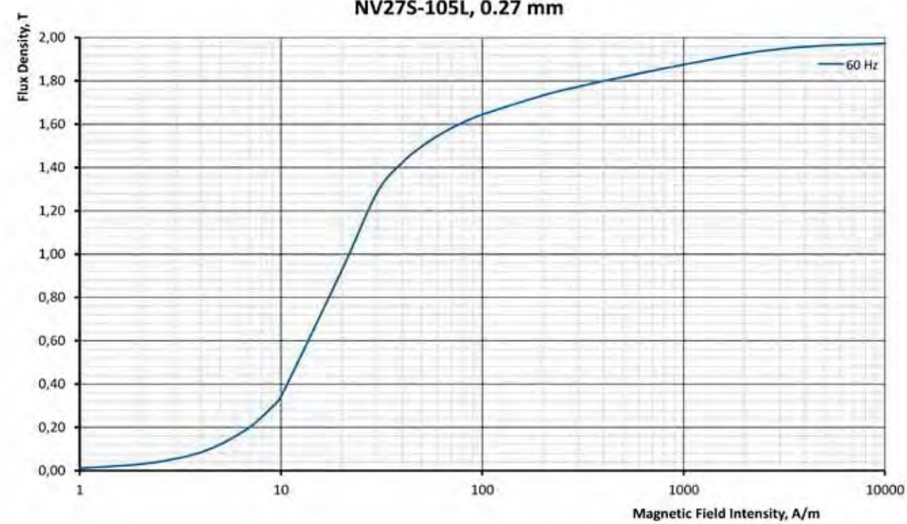
Magnetization curve NV27S-105L, 0.27 mm
