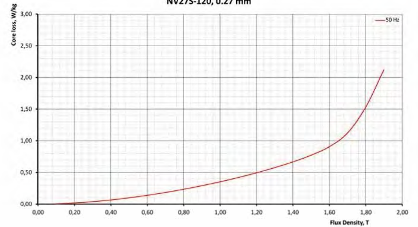
Specific core loss NV27S-120, 0.27 mm
