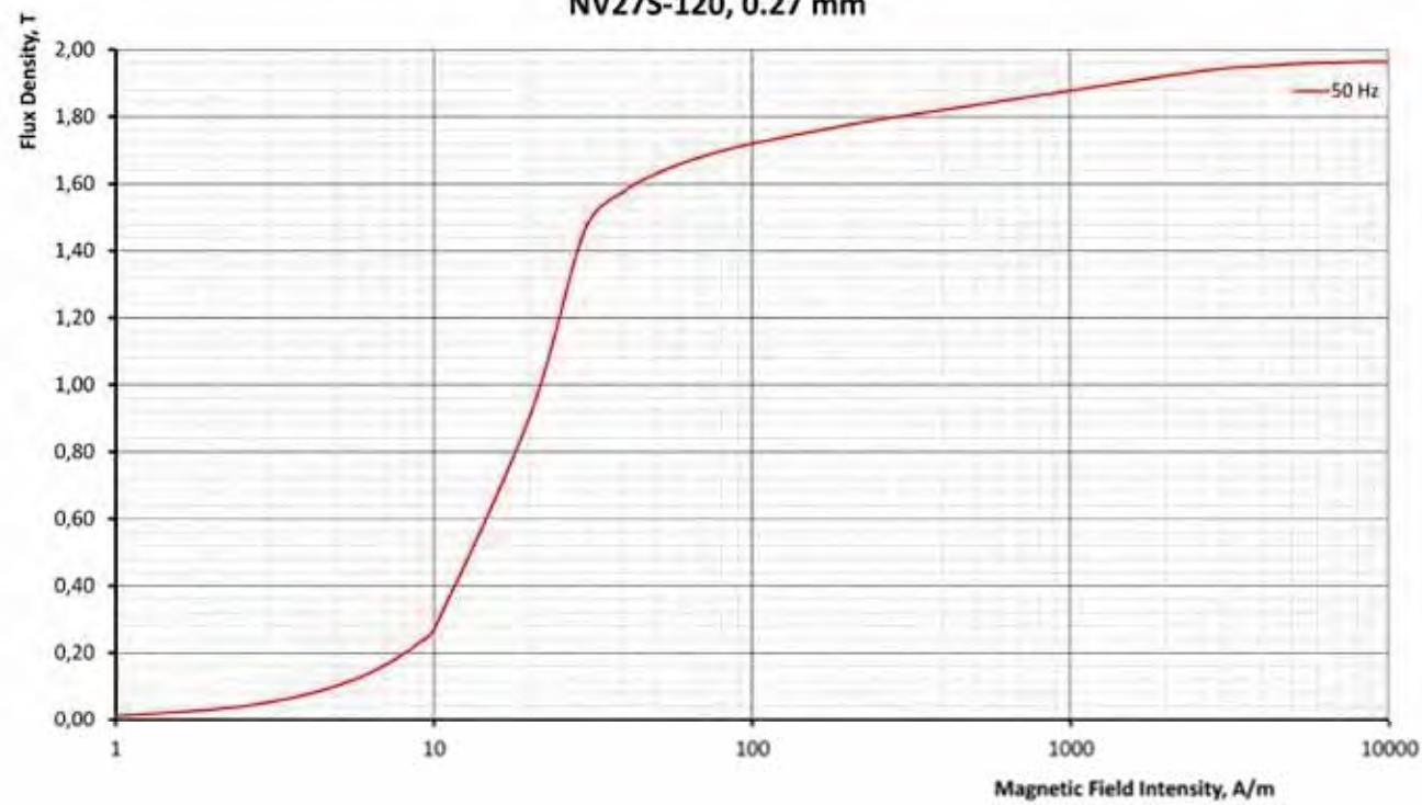
Magnetization curve NV27S-120, 0.27 mm
