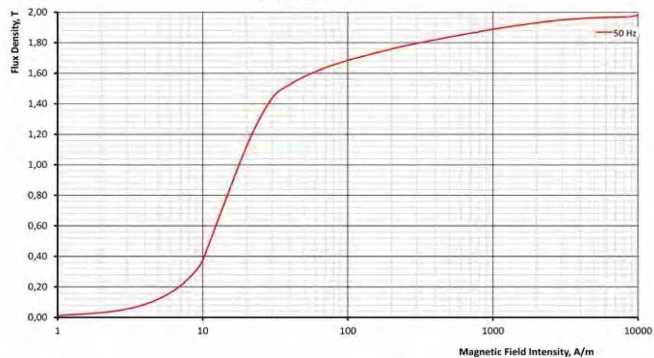
Magnetization curve NV23S-95L, 0.23 mm
